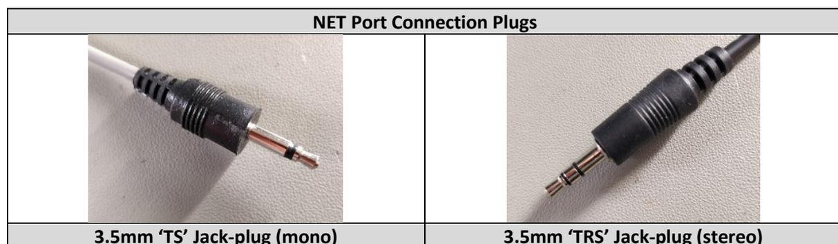
Each station is linked to the next in a daisy-chained/common-bus arrangement using either or both of the two (identical) NET sockets that lurk unobtrusively at the rear of your QL and Interface-1; the two stations that sit at the extreme ends of the chain **will only have one socket connected**, whereas each intervening station will have both occupied.
