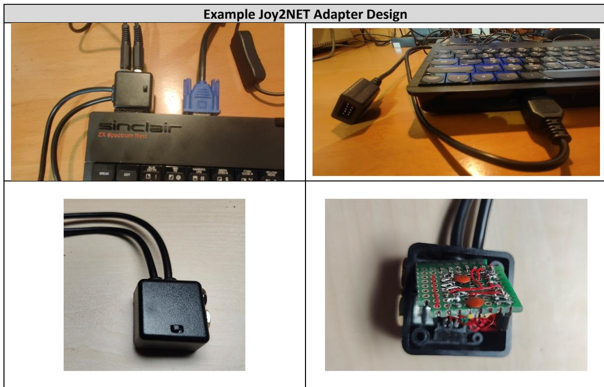
The Joy2NET adapter can be used alongside standard/passive Atari-style joysticks in port #1 if a pass-through cable/socket is added to the design (as shown). A standard Atari joystick is also supported in port #2 in any case.
