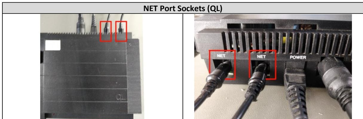
The most common situation of just two connected stations will therefore require only a **single** 2-core cable, leaving one NET socket disconnected on each station – it does not matter which of the two available sockets are used at each end.
