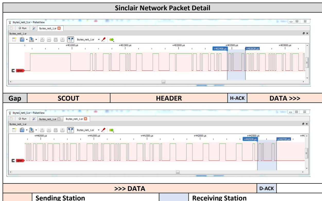
The sending station will **abort** the current transmission-cycle if any of the following conditions are detected:
