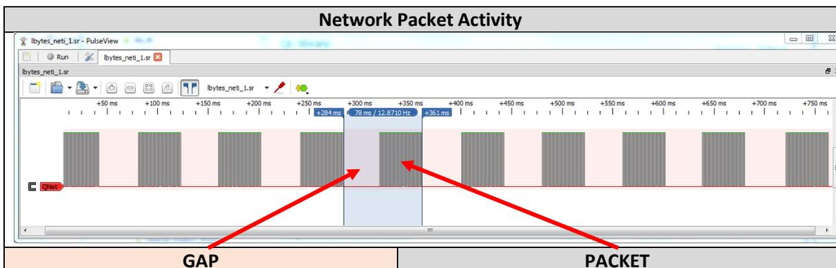
The sending station starts by 'listening' for a suitably long silence or **gap** indicating that the link is free, before placing a **scout** bit-pattern on the wire whilst simultaneously reading back the link state to ensure that no other station is also trying to claim the link.
